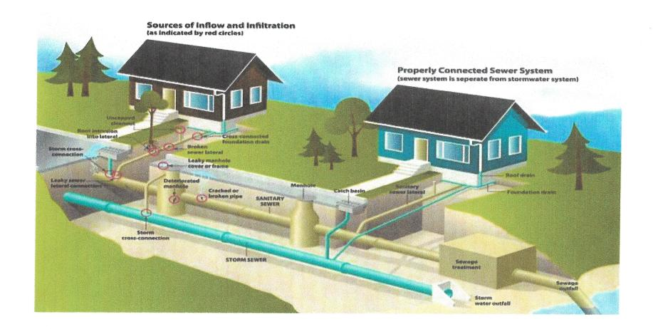
Proper Separation of Stormwater & Sanitary Lines
